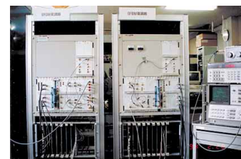
Figure 1: The first OFDM Modem for digital terrestrial broadcasting in Japan (1992)
