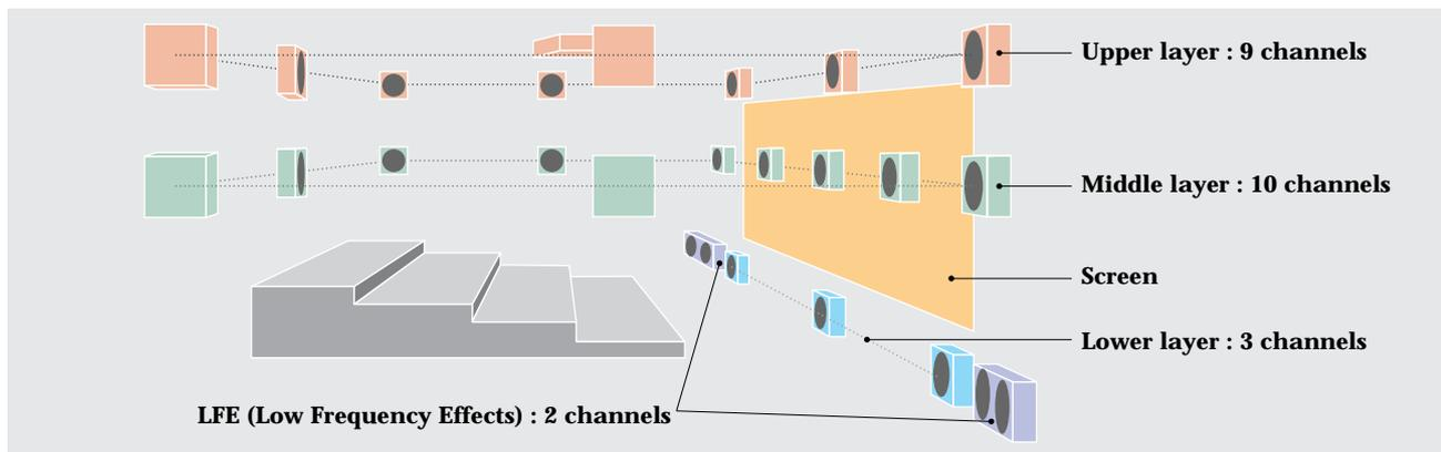
Figure 2: Outline of 22.2 multichannel sound system
