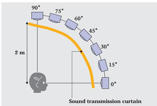
Figure 7: Loudspeaker positions used in experiment
