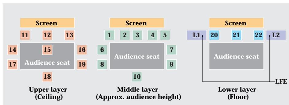
Figure 3: Loudspeaker arrangement of 22.2 multichannel sound system
