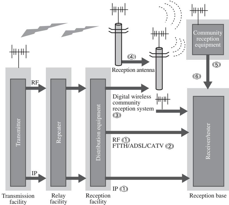
**Figure 8. IP Multicast Signal Transmission**
