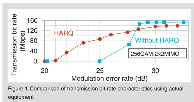
Figure 1. Comparison of transmission bit rate characteristics using actual equipment
