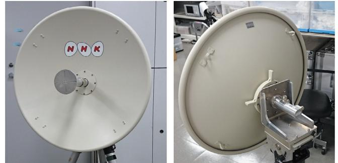
Figure 2. Dual-polarized parabolic antenna with splash plate (left: front, right: back)
