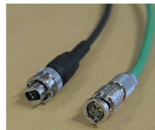
Optical cable for UHDTV production system interface (left)
