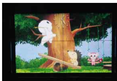
Example of video image reproduced on 0.285 mm pixel-pitch ultra-high-resolution 7-inch diagonal PDP with SrCaO protective layer (Exhibited at the 2008 STRL Open House)
