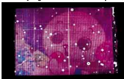
Figure 3. Liquid crystal film display driven by organic TFTs (160×120 pixels)
