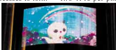
Figure 1. Liquid crystal film display driven by polycrystalline silicon TFTs (128×72 pixels)
