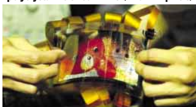
Figure 2. Flexible organic EL display driven by organic TFTs (213×120 pixels)
