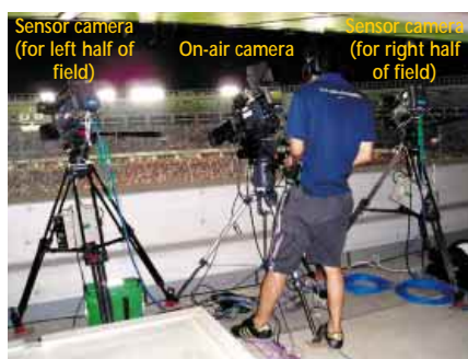
Figure 2: On-air camera and sensor cameras
