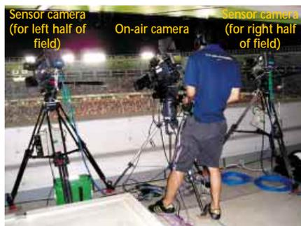
Figure 2: On-air camera and sensor cameras
