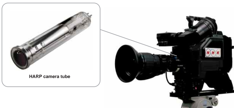
Figure 9: Ultra-high-sensitivity hand-held HDTV HARP camera
