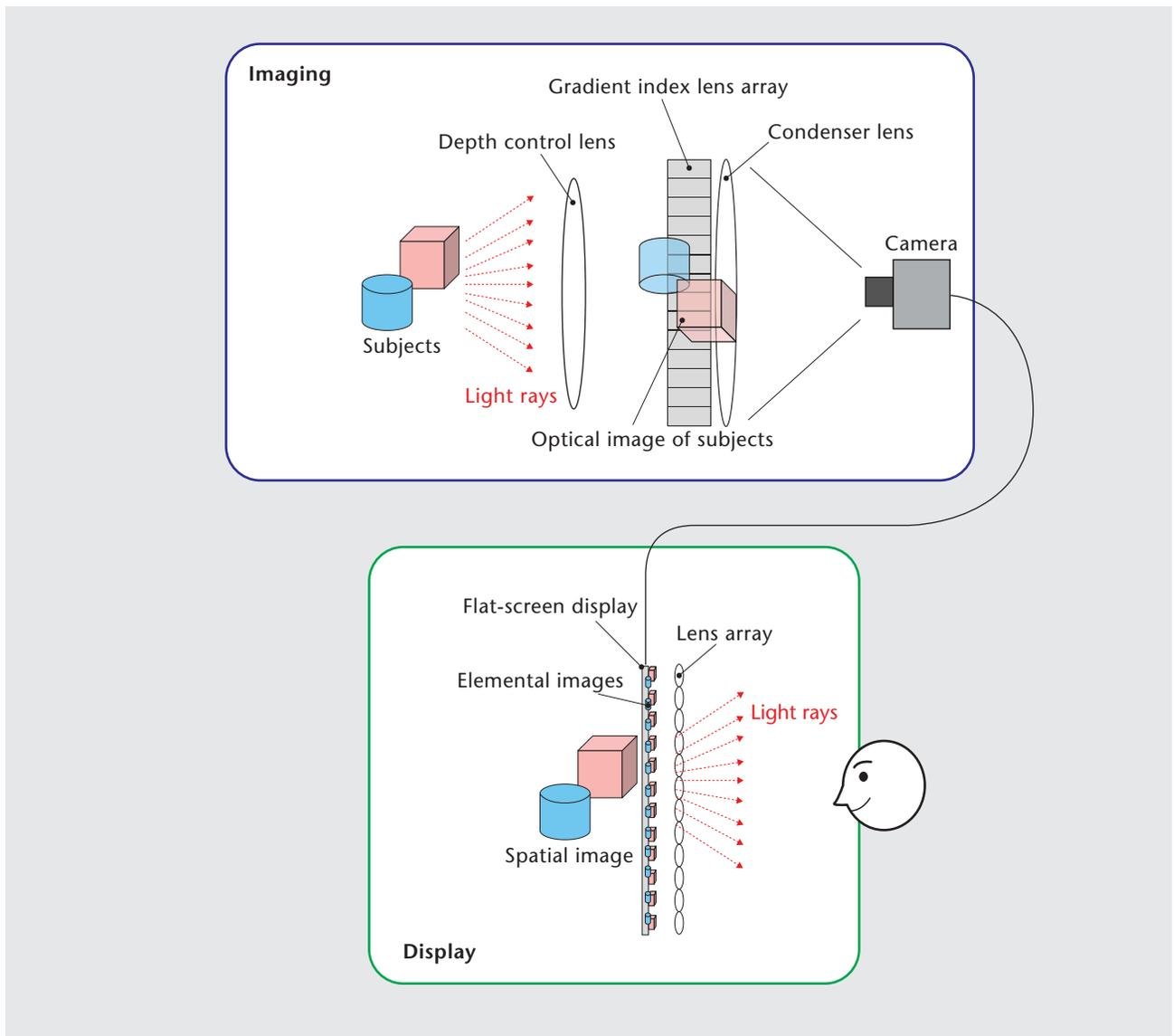
**Figure 3: 3D TV system implemented by integral method**
