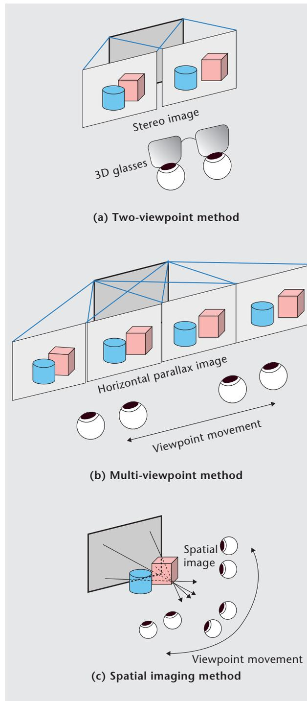
Figure 2: Different stereoscopic vision methods
