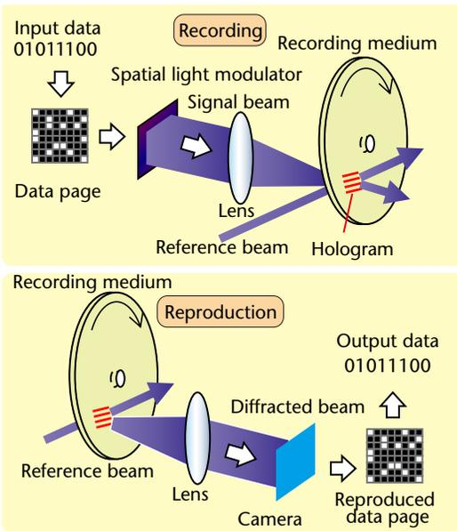
Figure 1: Holographic memory recording/reproduction principle
