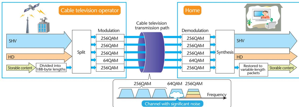
Figure 1: SHV cable television broadcasting using multiple carrier-waves
