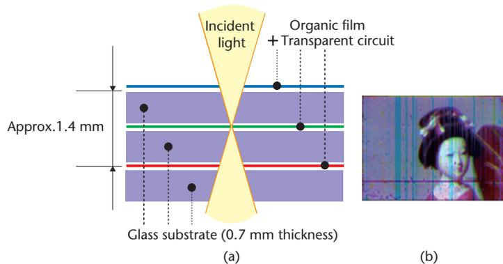
Figure 1: (a) Structure of organic image sensor for principle verification (b) Output image
