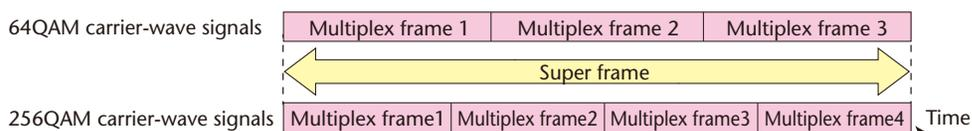
Figure 2: 64QAM and 256QAM signal synchronous combination
