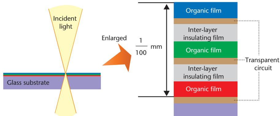
Figure 2: Structure of continuously-stacked organic image sensor
