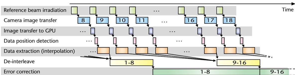
Figure 2: Pipelined parallel processing for reproduced signals (number indicates the processing order of individual data page sets)
