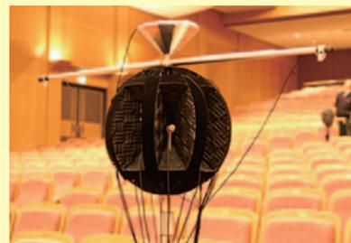
Picture 1: Compact sphere-shaped 22.2 audio one-point microphone
