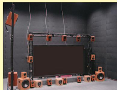
Picture 3: 22.2ch sound reproduction system for 145-inch PDP
