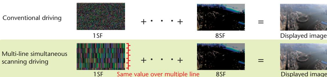
Figure 2: Multi-line simultaneous scanning method
