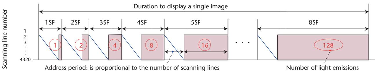
Figure 1: PDP driving scheme
