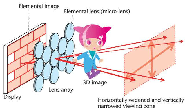
Figure 3: Viewing zone of new integral 3D TV with expanded horizontal viewing zone
