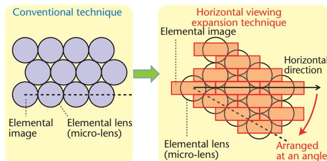
Figure 2: Elemental lens and elemental image arrangement
