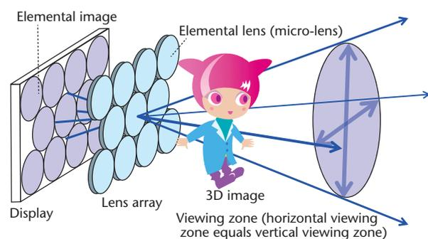
Figure 1: Viewing zone of conventional integral 3D TV
