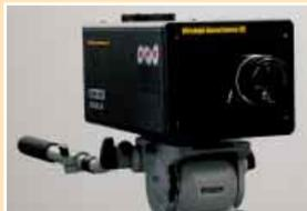
We are making advances on camera systems that can capture clear images of high-speed phenomena that cannot be perceived with the naked eye or ordinary cameras. Our latest ultrahigh-speed, high-sensitivity CCD and its camera system has a maximum shooting speed capability of one million frames per second.
