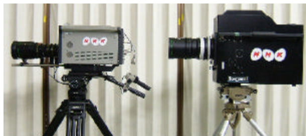
Figure 1. External view of two 8k x 4k pixels camera heads. Previous prototype (right:2.5-inch CCD) and newly developed (left:1.25-inch CMOS).
