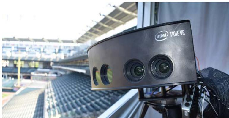
**True VR creates its VR content through the placement of multiple cameras so they surround the playing field. Delivery of multi-view video is also possible (photo supplied by Intel).**
